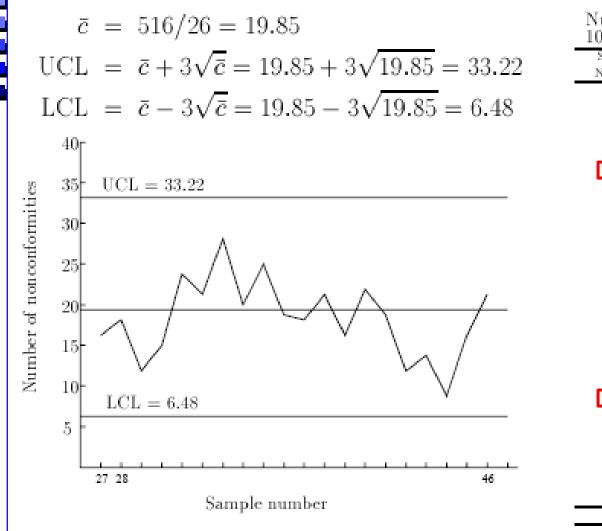
Number of defects in samples of 100 printed circuit boards
